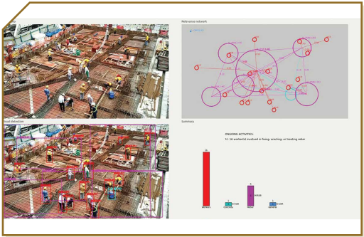
A computer vision-enabled digital twin for construction resource and progress management 施工資源與進度管理數字孿生技術研究
