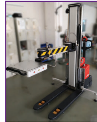
Smart Lifter/Transporter for Object Handling in Confined Spaces 適用於擠迫環境的智能起重機/運輸機器
