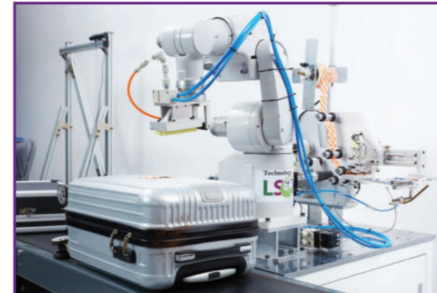
Smart Robot Hand and Eye Co-ordination Enabling Technologies for e-Commerce Warehouse Management 應用於電子商貿倉庫之智慧型手眼協調機械臂定位系統
