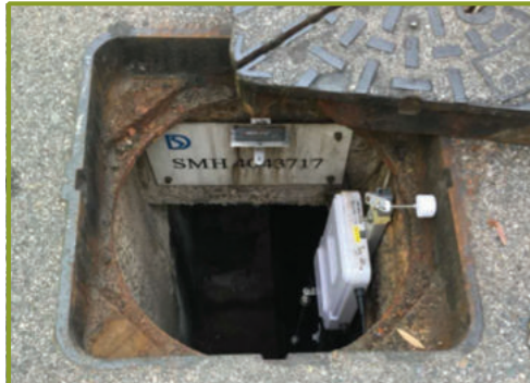
An Integrated Sensor Module and Ubiquitous Wireless Network for Smart Drainage System 結合無線傳感模組及網絡的智能渠道管理系統
